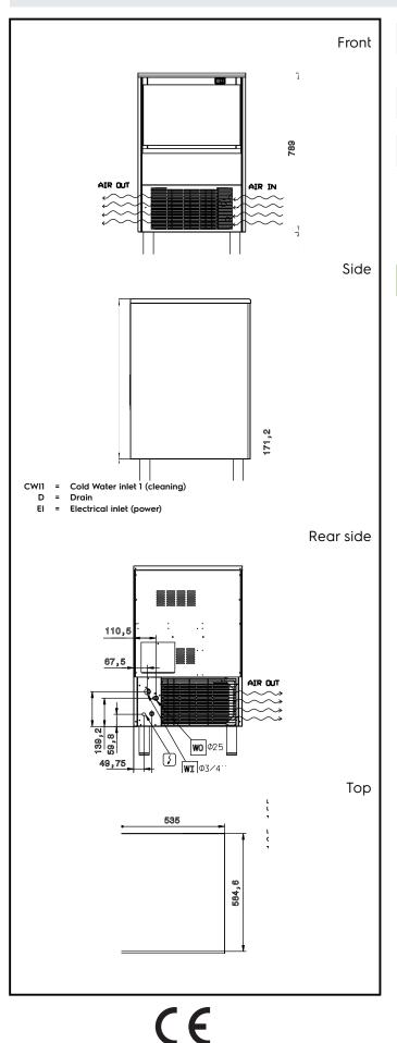
Supply voltage: 220-240 V/1N ph/50 Hz Electrical power, max: 0.37 kW Capacity: Bin capacity: 25 kg Key Information: External dimensions, Width: 535 mm 595 mm External dimensions, Depth: External dimensions, Height: 894 mm Net weight: 56 kg Output: 56 kg/day Kind of cube: Ice Cube 22 g **Sustainability** R290 **Refrigerant type:** Refrigerant weight: 65 g Water consumption: 30.5 lt/hr
